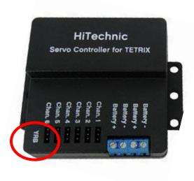
Figure 11: YRB Marking on the Servo Controller.
