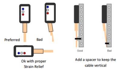
Figure 6: Samantha Module placement tips.
