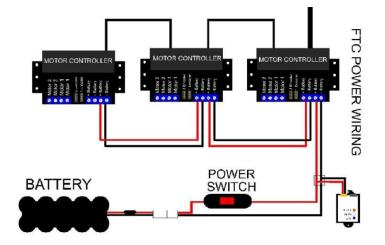
Figure 16: A simple wiring diagram.
