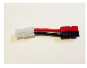
Figure 24: Tamiya/Powerpole Adapter.
