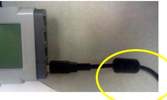
Figure 9: Ferrite choke in use on a USB cable
