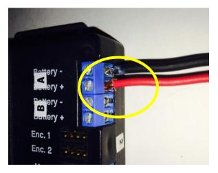
Figure 7: Try to avoid stray strands of wire when connecting to the Motor Controller.
